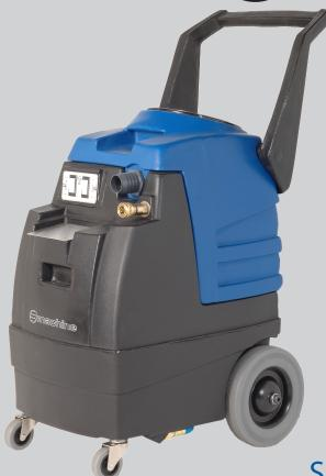
The E600 is a compact high performance extractor featuring 6 gallon solution and recovery tanks, a high output 3 stage vacuum motor and 150 PSI demand solution pump. Complete with fold down handle making it easy for transportation in almost any vehicle. Available with or without internal inline heater.
