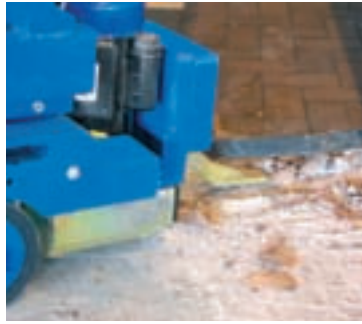
Angle Attachments angle the cutting head or carbide shank to where the material comes up the easiest
