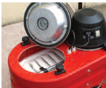
Motors are easily removed for service
