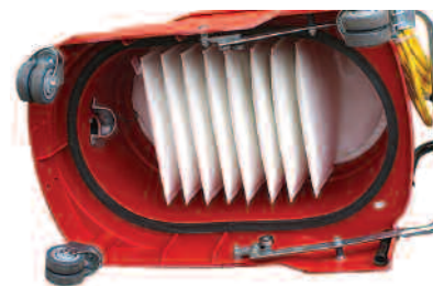
Metal frame supports filter element
