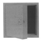
For use in wall and ceiling applications including drywall, masonry and suspended acoustical ceilings. Features 16-ga. steel frame with 20-ga. door panel, 2" mineral fiber insulation for reduced sound transmission, continuous hinge with stainless steel pin, and factory installed masonry anchors. Self-latching. UL and CUL class B fire rated.
