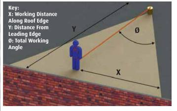
For example, if the anchorage connector is 6' from the leading edge (Y), the working distance (X) is 8' in each direction from the perpendicular, which translates to a 53° working angle.
