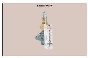
Regulator Kits are available as optional extras for both Rate-Master® Flowmeters and Visi-Float® Flowmeters models. This view shows Model VFA Visi-Float® flowmeter with integrally connected constant differential pressure regulator. Recommended for use where inlet air pressure fluctuates widely and constant flow is required.
