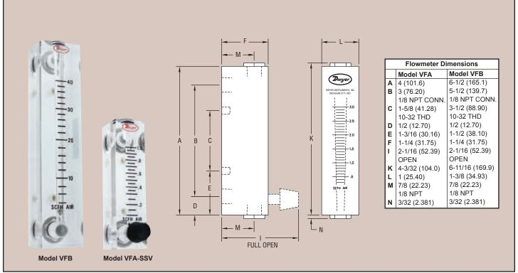
The Visi-Float® flowmeter bodies are cut and precision machined from solid, clear acrylic plastic blocks. This construction not only produces a handsome finished product, but permits complete visual inspection. As a result, the Visi-Float® flowmeters are especially popular for medical and laboratory equipment applications.
