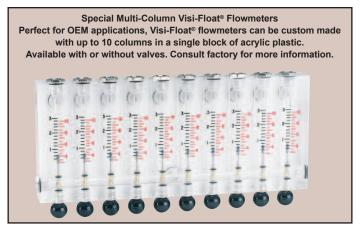
**OEM Specials** — Special flowmeter designs can be supplied to meet a wide range of requirements and specific applications. These include: on-off plunger and push-to-test valves, special gas or fluid calibration, special ranges, scales, name brand or other identification. Pointer flags can be furnished for instant visual reference. For specific information, please supply an outline of your requirements.
