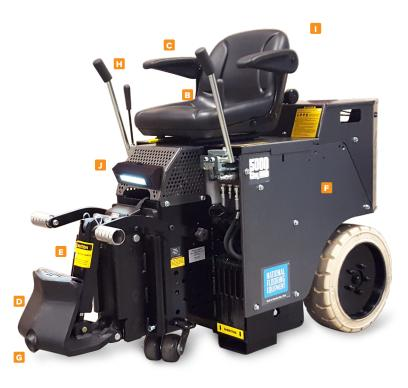
The 5000 is a compact, ride-on oor scraper designed with a low-pro le frame that increases ease of transport and maneuverability on the job.
