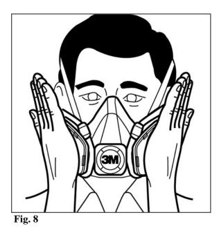
Note: Before assigning any respirator to be worn in a contaminated area, a qualitative or quantitative fit test must be performed per OSHA Standard 1910.134 or CSA Standard Z94.4.
