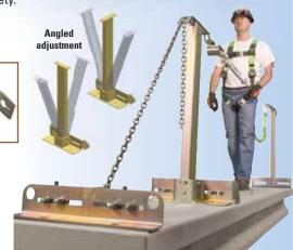
Complete system includes stanchions, tie-back brackets, chain connectors, slider brackets, energy absorber(s), line tension indicator, turnbuckle, cable and hardware. Attach to rebar, coil inserts or concrete expansion bolts.
