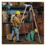
A secondary fall arrest system is recommended
