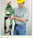
Step 2 If chest, leg and/or waist straps are buckled, release straps and unbuckle at this time.
