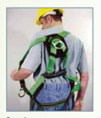
Step 3 Slip straps over shoulders so D-ring is located in middle of back between shoulder blades.
