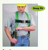
Step 6 After all straps have been buckled, tighten all buckles so that harness fits snug but allows full range of movement. Pass excess strap through loop keepers.
