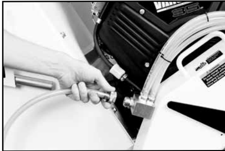
Fig. 6 Unscrew Hose Fitting
