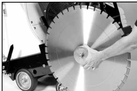
Fig. 11 Slide Outer Flange in place
