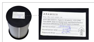
The HEPA filter is individually tested and certified to be 99.97% efficient at .3 microns according to IEST-RP-CC001 test requirement.
