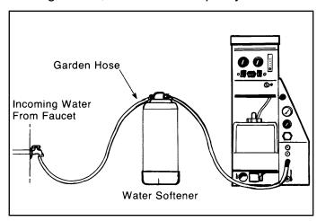
Figure 1-2. Configuration of Water Softener and CDS
