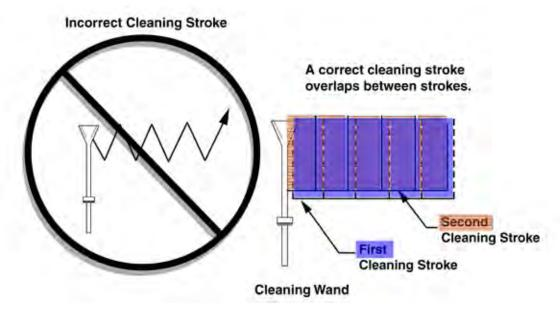
Figure 2-2. Cleaning Stroke Procedure
