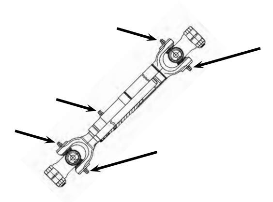
Figure 10-1. Zerk Fittings on Drive Shaft (Chevy and Ford)
