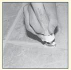
▲ Turbo Stick grout sealing tool
