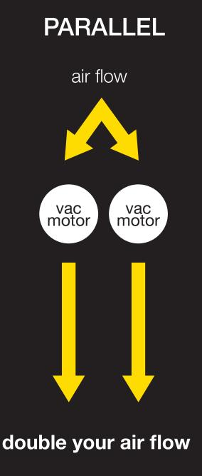
The new Nautilus with AirFlow+ allows you to customize your vacuum configuration. Run the vacuums in Series to increase your lift by 60%, or double your air flow by running in Parallel.
