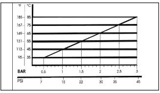
Naturally, if the application allows for feeding the pump with 45 psi (3 bar) even at low temperatures (for example:  $115^{O}F/45^{O}C$  the life of the wet end of the pump will be even longer.
