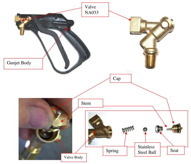
• Examine the Cap, Spring, Seat and Steel Ball for signs of wear or pitting. Replace Spring as needed. Replace the Seat o-ring. Replace Steel Ball as needed. Remove Stem from Cap and replace seals as needed. If the valve body, cap or seat is worn or damaged, replace the whole valve (NA033).
