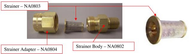
**Quick Connect** – The inlet quick connect may be damaged or obstructed and not allowing the proper water flow through. Clean or replace the quick connect as needed. (**AH102B**)
