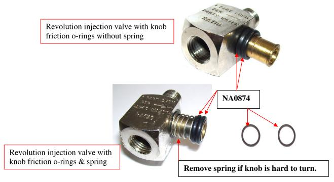
The Revolution Injection Valve can be repaired and recalibrated in the field. The Stem Assembly (NA0869) can be replaced on the Revolution Injection Valve. The stem assembly is included in the major repair kit (NA0849R). The seat in the new valve is more resistant to the damage caused by over tightening the stem.
