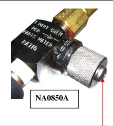
Remove screw to recalibrate
